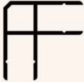
SIDING KENAR KAPAMA (SIDING EDGE CLOSURE)
